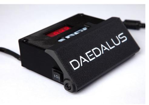
Before you get started, always make sure the direction switch on the Speed Controller is in the middle (neutral) position, or else the wheel will attempt to start when you're not ready. Please read the directions for using the Speed Controller, for more in-depth information.
