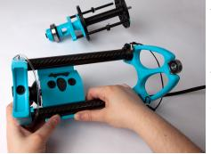
Install the tension belt at the front, over the flyer groove. Please note that your direction switch will be opposite in Irish as compared to Scotch tension (meaning that I is S and II is now Z). You will need to slide the motor mount in a rocking motion, until it aligns under the small bobbin whorl at the rear of the bobbin and the other end of the chassis. Verify this visually from the side to ensure the drive belt is parallel with the rear frame.
