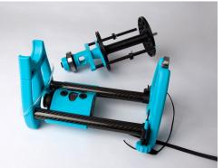
Irish tension provides more takeup, or pulling in of the yarn, than Scotch tension. Changing to Irish tension is as easy as removing the flyer, tension belt, and motor drive belt.
