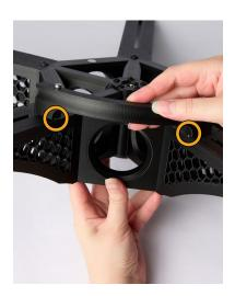
Line up the ends of the **Bolts** on the **Whorl Piece** to holes on the arms at the back of the **Hub**, then screw into place with **2.5** mm Allen Wrench.
