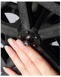
Place the **Front Axle Spacer** onto the **Axle** with the tapered side facing the **Bearing** in the **Hub**.
