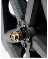
When the **Axle** has been pushed in all the way and all parts are pushed in fully, there should be about **4 mm** (a bit over 1/8") of extra axle in front. If there is more showing, then the axle is not pushed into the **Top Plate** all the way.
