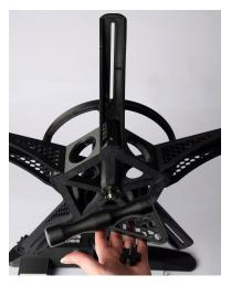
Screw (5) **Arm Posts** onto the ends of the **Arms** using the provided (5) **Arm Post Knobs**.
