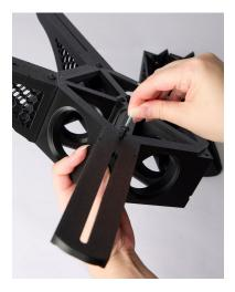
Using (4) **M5x16 Bolt** and the **3 mm** Allen Wrench, attach the other (4) **Arms**. A small amount of creaking should be expected.
