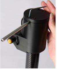
Tighten the (4) M5x16 Bolts by one full turn in the Top Plate, using a 3 mm Allen Wrench. Tighten down enough so the Axle is secured. The Top Plate will not fit flush the the edges. Tug on the axle to ensure it doesn't move.
