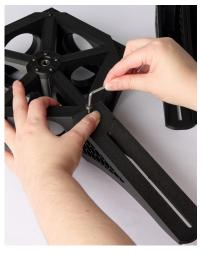
Place an **Arm** on the **Hub**. Using (1) **M5x16 Bolt** and the **3mm** Allen Wrench, secure the Arm to the back of the Hub.
