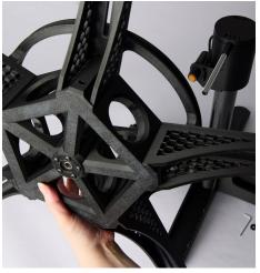
Pick up the **Head** and slide it onto the **Axle** with the **Sensor Magnet** and **Whorl** side facing the **Top Plate**.
