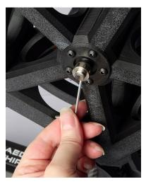
Place the **Lock Ring** onto the **Axle**. If it doesn't want to go on, ensure the **Grub Screw** is backed out enough. Push the Lock Ring on and secure the grub screw that's already in place using the **2 mm** Allen Wrench.
