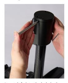
Insert **Axle** into the hole in the side of the **Top Plate**. Use your hands to apply even force from both sides to ensure the **Axle** goes in all the way.
