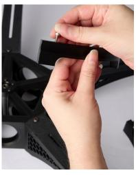
Pick up a **Whorl Piece** and place **M3x30 Bolts** in both holes. Using your fingers, screw the bolts through the piece far enough that they peek out the other end of the hole.
