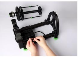
Irish tension provides more takeup, or pulling in of the yarn, than Scotch tension. Changing to Irish tension is as easy as removing the flyer, tension belt, and motor drive belt.
