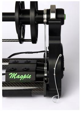
drive the flyer and the tension belt provides resistance to the bobbin, allowing yarn to wind on. In Irish tension, it's the opposite: the bobbin is led by the motors. Because of this feature, you will need to make sure the motors and the pinion pulleys are properly aligned, directly underneath the appropriate whorl before spinning.
